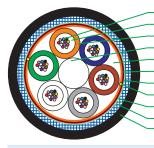
Primary Coated Fibre Tube Filling Compound Loose Tube(s) Central Strength Member .Cable Filling Compound Peripheral strength member .Core Wrapping Rip Cords Water blocking media under armour Armouring (T for steel = 0.15 mm Nom) Outer Sheath (T = 1.5 mm Min)
